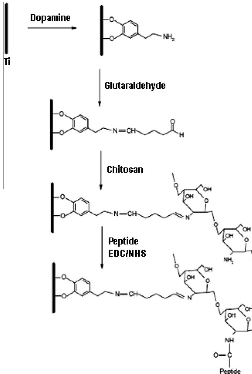
**Fig. 3.** Immobilization of chitosan and RGD peptide on Ti substrates. Amine coupling agents for covalent binding of RGD peptide: EDC, 1-ethyl-3-(3-dimethylaminopropyl) carbodiimide; NHS, N-hydroxysuccinimide. Taken from [78].
