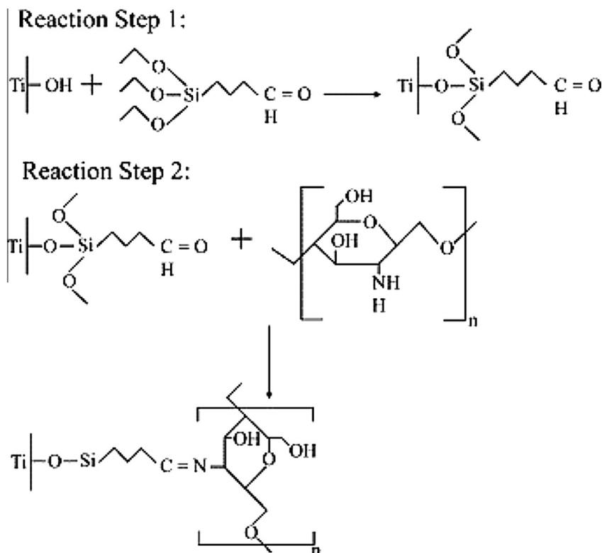
Fig. 5. Reaction steps involved in the binding of chitosan to titanium substrates via silanation with triethoxysilylbutyraldehyde (TESBA): (1) TESBA deposition; (2) reaction of TESBA with chitosan. Taken from [83].
