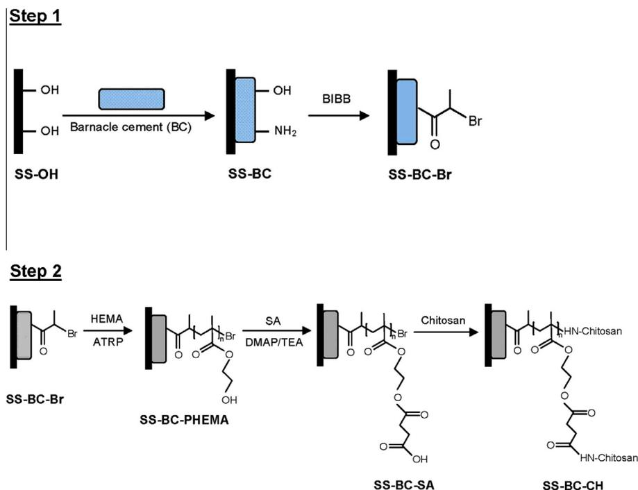
**Fig. 7.** Chitosan grafting on stainless steel (SS) surface via poly(2-hydroxyethyl methacrylate) (PHEMA) brushes. Step 1. Immobilization of alkyl bromide ATRP (atom transfer radical polymerization) initiator via barnacle cement (BC). BIBB, 2-bromoisobutyl bromide. Step 2. Surface-Initiated ATRP of 2-hydroxyethyl methacrylate (HEMA) and chitosan (CH) immobilization. DMAP, 4-(dimethylamino)pyridine; TEA, trimethylamine; SA, succinic anhydride. Adapted from [90].
