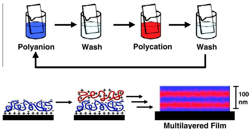
**Fig. 9.** Layer-by-layer deposition of oppositely charged polyelectrolytes on surfaces. (Top) Fabrication proceeds by iterative dipping of a substrate into dilute aqueous solutions of cationic and anionic polymers. (Bottom) Electrostatic interactions guide the assembly of multilayered polyelectrolyte assemblies. Taken from [94].
